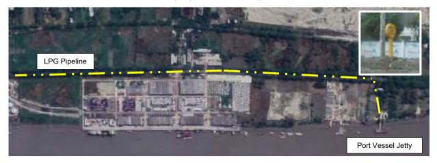
Figure 2-17: Arrangement of LPG Pipeline [Google Earth 2019]
