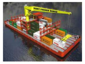
Figure 10-8: Technical concept rendering for container mid-stream handling
