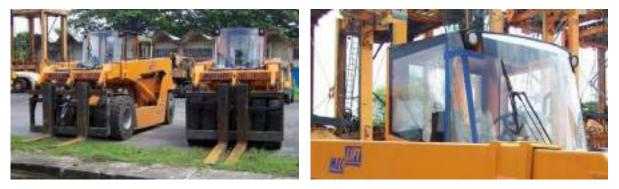
Figure 2-46: Damaged Windows at both MECLIFT Reach Stackers [Consultant]
